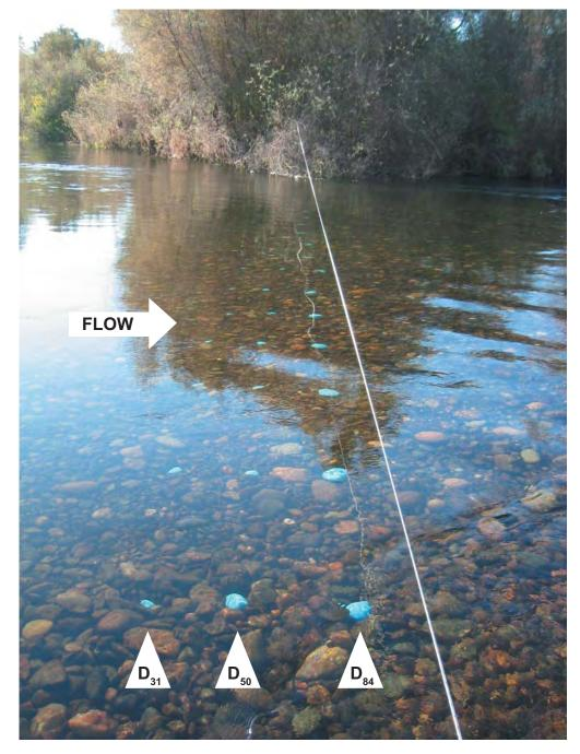
Figure 12. Example of marked rock placement at riffle crest Patch 1.
