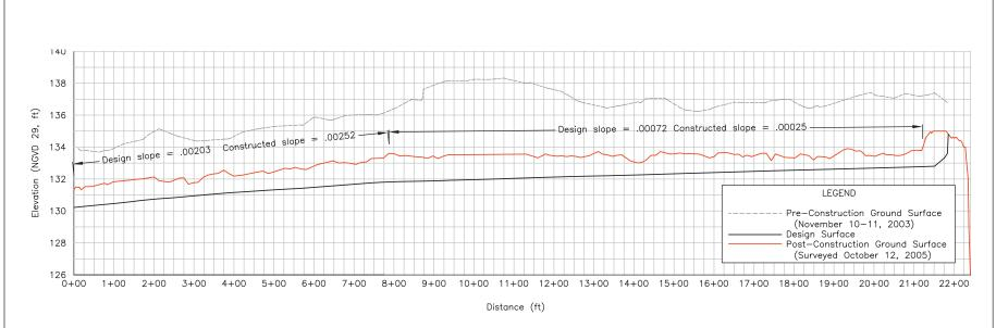
Figure 17. High flow scour channel existing, design, and as-built longitudinal profile. Longitudinal stationing for high flow scour channel is shown on Figure 15.
