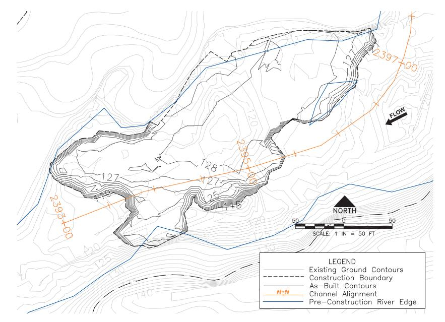
Figure 22. Existing and as-built contours at Patches 5 and 6.
