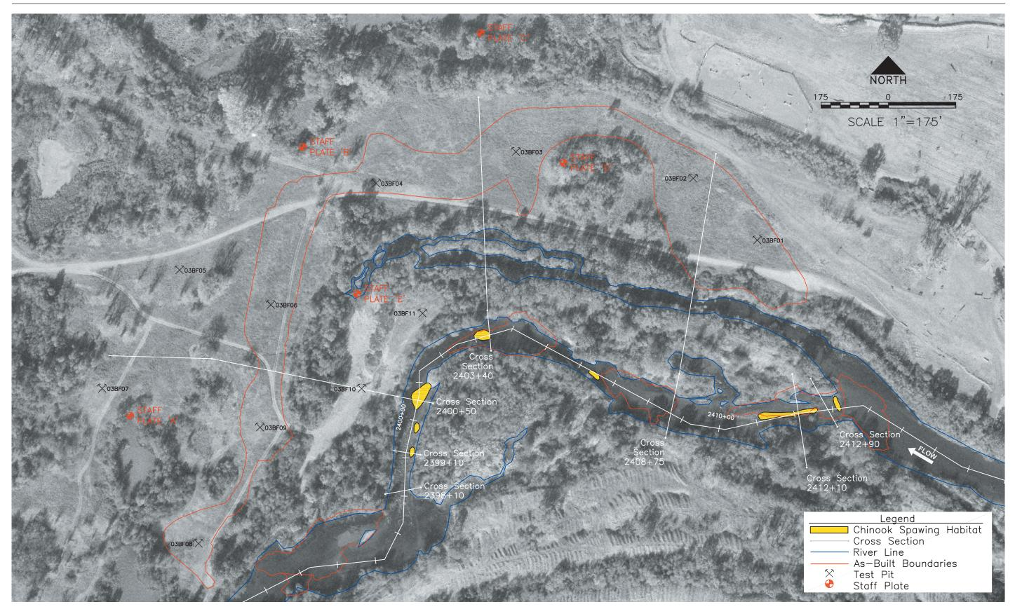
Figure 10. Pre-construction cross sections, ground water monitoring sites, material test pit locations, and Chinook spawning habitat areas.
