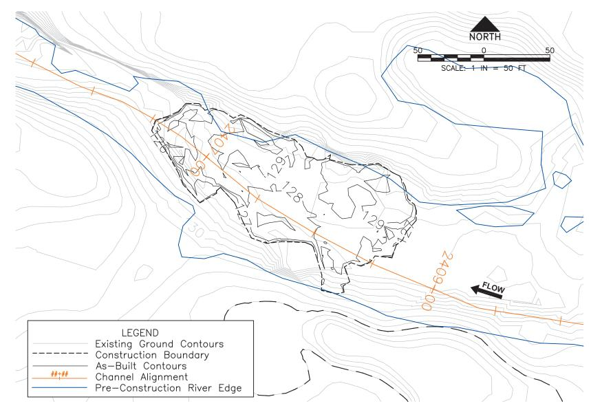
Figure 20. Existing and as-built contours at Patch 3.
