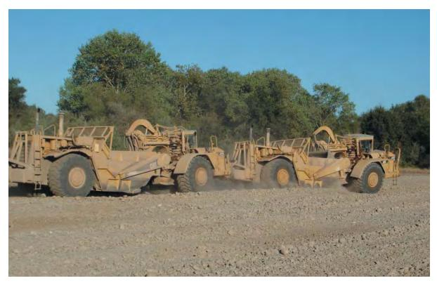
*Figure 2. Two Caterpillar 627G scrapers working in tandem while excavating material from floodway (Photograph courtesy of Friends of the Tuolumne).*
