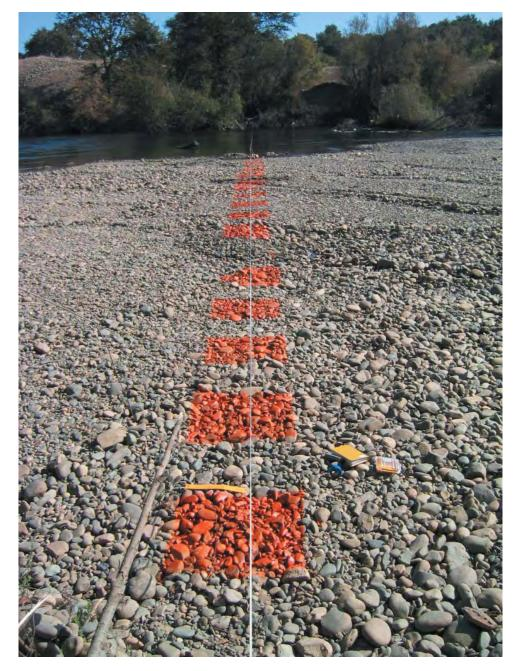
Figure 14. Example of 2 ft x 2 ft paint patches set at Patch 6.
