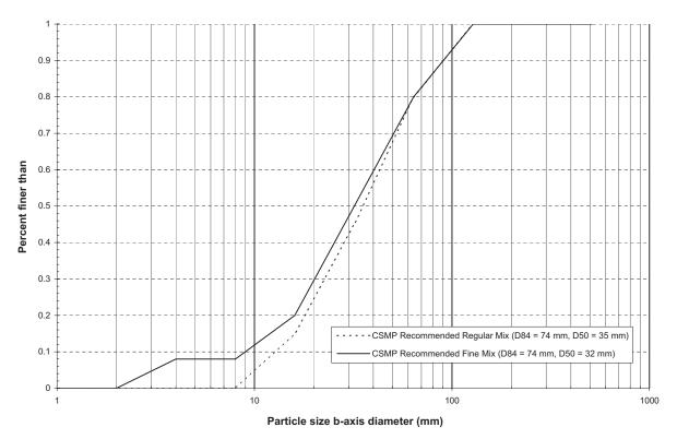
Figure 24. Recommended mixes for instream gravel augmentation projects (from McBain & Trush, Inc., 2004.
