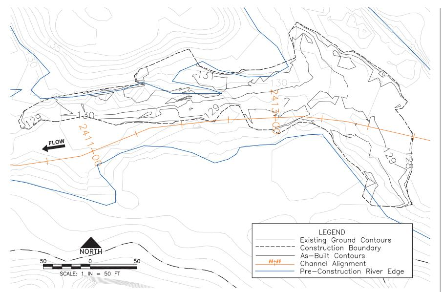
Figure 19. Existing and as-built contours at Patches 1 and 2.
