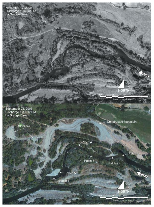
Figure 29. Pre- and post-construction aerial photographs for Bobcat Flat RM43 Phase I project area.
