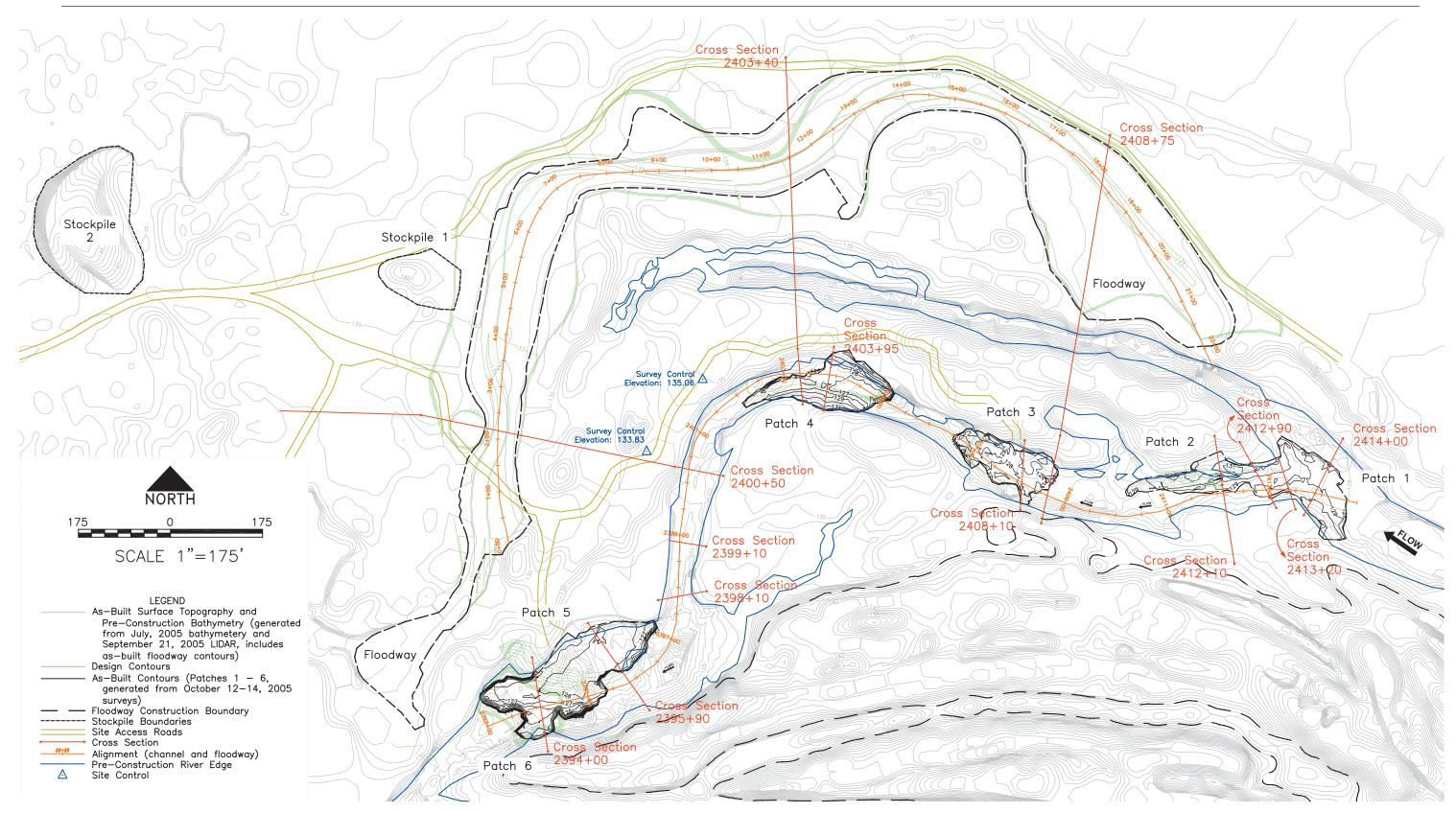
Figure 15. Bobcat Flat planform map of existing, design, and as-built contours.
