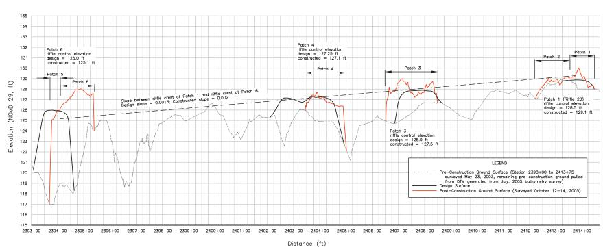
Figure 23. Longitudinal profile of existing, design, and as-built ground surfaces using pre-construction alignment. Longitudinal stationing and channel alignment location is shown on Figure 15.
