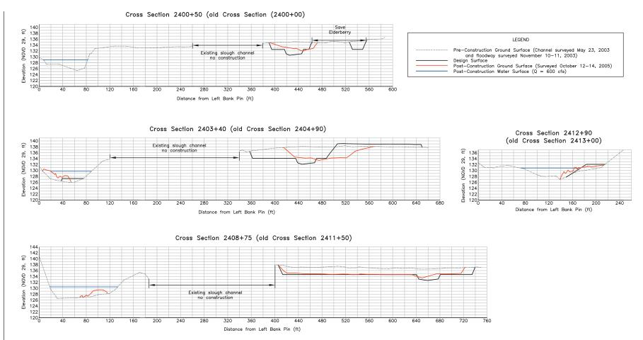
Figure 16. Bobcat Flat existing, design, and as-built cross sections. Cross section locations are shown on Figure 15.
