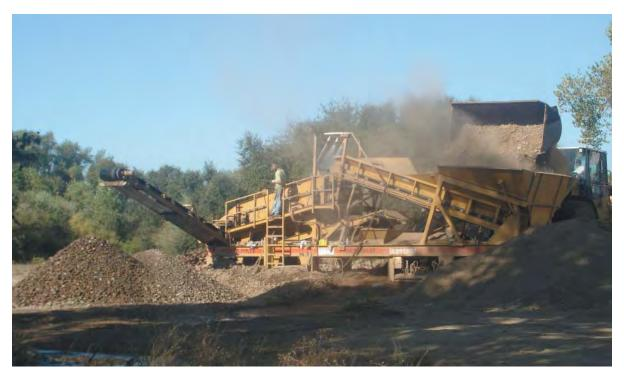
*Figure 6. Resulting <sup>1</sup>/<sub>4</sub> to 5 inch sieved washed coarse sediment ready for placement in channel (Photograph courtesy of Friends of the Tuolumne).*
