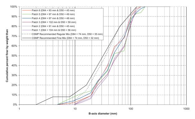
Figure 26. Plotted summary of results for bulk samples taken at each of the constructed patches. Bulk sample locations are shown on Figure 11.
