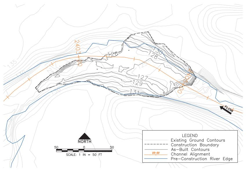
*Figure 21. Existing and as-built contours at Patch 4.*
