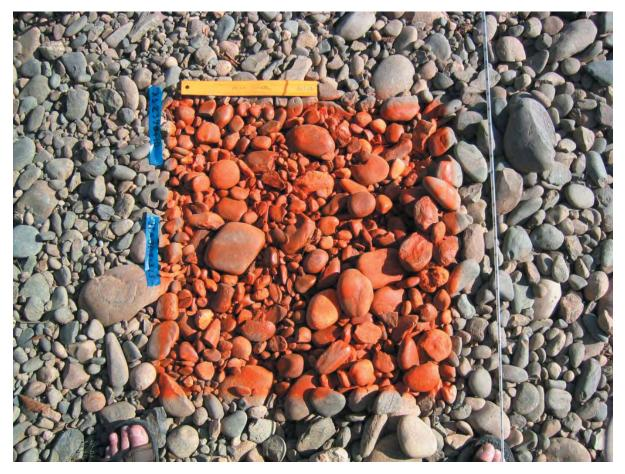
*Figure 13. Example of a single 2 ft x 2 ft foot paint patch monitoring photograph.*
