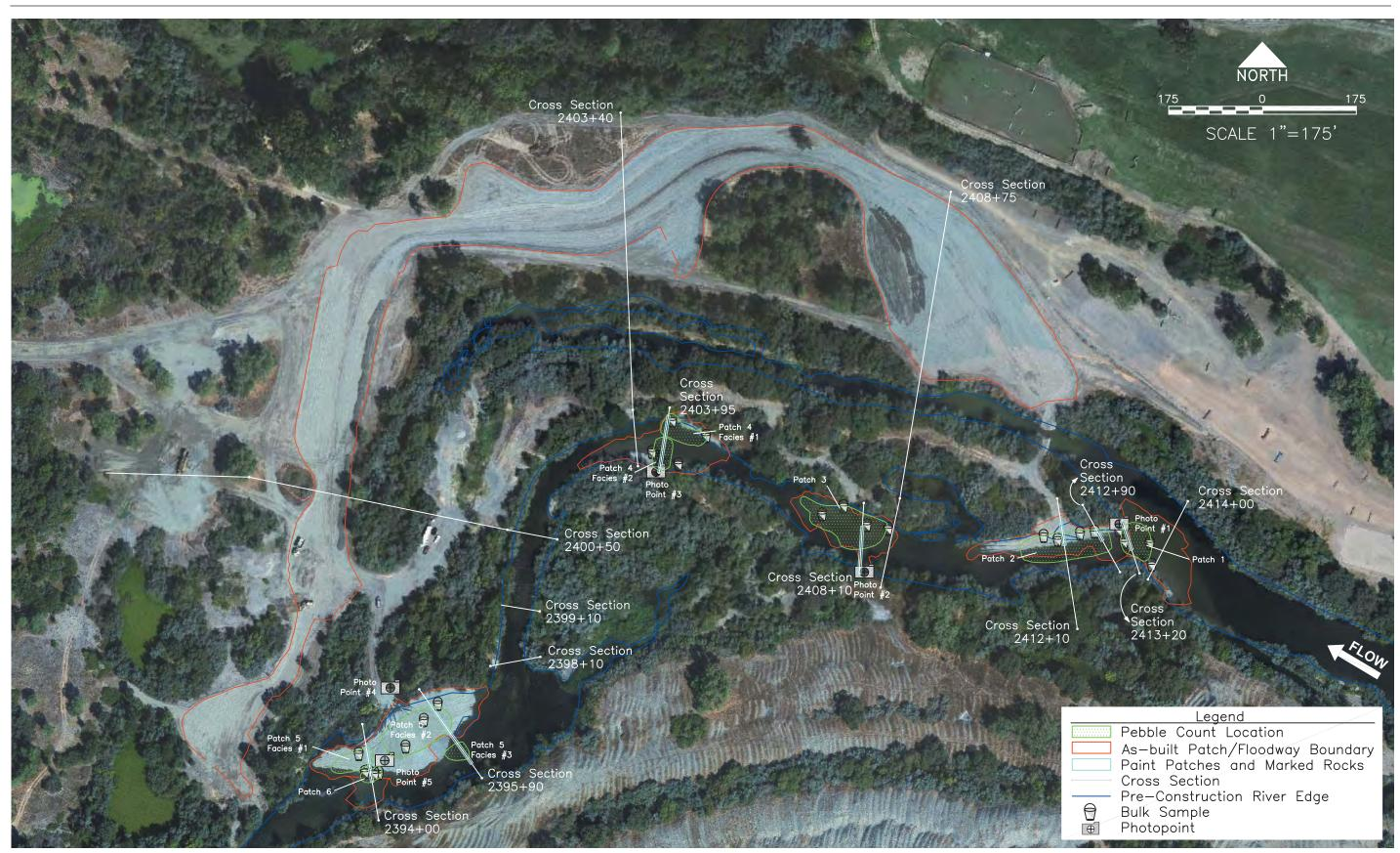
Figure 11. Post-construction cross sections, photo points, bulk sample, pebble count, and marked rock deployment locations.
