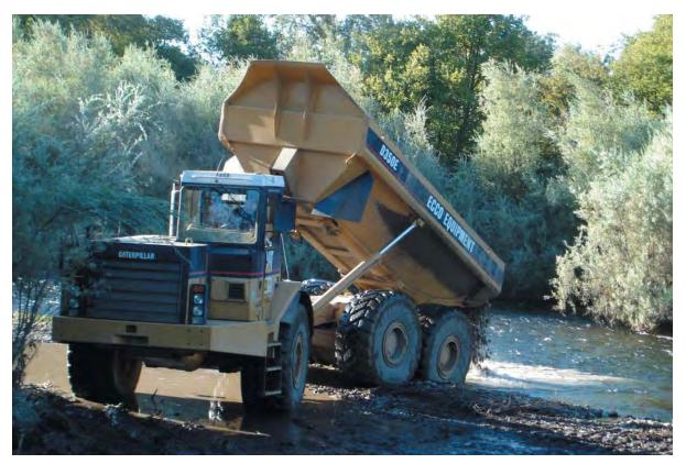
*Figure 7. Caterpillar D350E (21 yd<sup>3</sup>) articulated truck dumping coarse sediment at Patch 2 (Photograph courtesy of Friends of the Tuolumne).*
