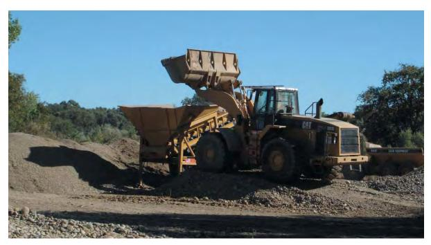
Figure 4. Caterpillar 980G front end loader placing raw material from stockpile into hopper for sieving and washing (Photograph courtesy of Friends of the Tuolumne).
