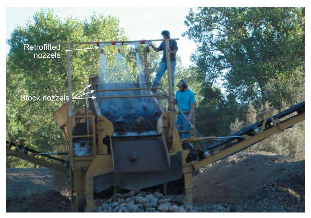
Figure 5. Sieving and washing plant consisting of Construction Equipment Co. (CEC) Screen-It, diesel powered screener, retrofitted with an additional washing system that sprayed water through three fire nozzles aimed at the screen (Photograph courtesy of Friends of the Tuolumne).
